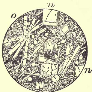
Fig. 34. — Nepheline-Trachyte (Phonolite). Brůx, Bohemia. \times 35 . n , Nepheline, in rectangular and hexagonal sections, showing zoning. o , Orthoclase (sanidine), in numerous needles and in stellar groups. Dark green patches (soda-pyroxene) occur in the hemicrystalline groundmass.
